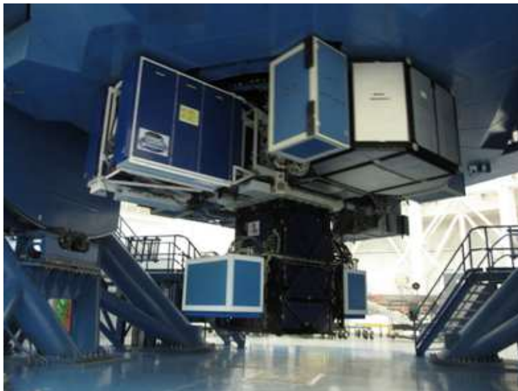
Figure 1: GPI (bottom) mounted on the Cassegrain mount of the Gemini South telescope, Chile.
