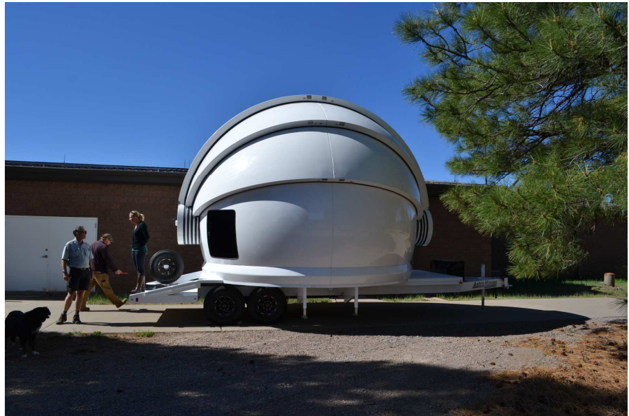
Figure 2. The first Astro Haven Enterprises (AHE) 16-dash-1 trailer-mounted ‘Enclosure-Transporter’ domes after delivery to NPOI from AHE.
